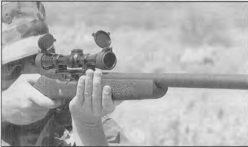
AWC Systems Technology's 10/22 Ultra system represents an advanced concept in a sound-suppressed .22 LR rimfire semiautomatic rifle. As the suppressor's housing is only 1 inch in diameter, the appearance is that of a heavy-barrel target rifle.
